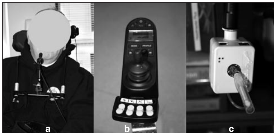
Figure 4 Control interfaces for EPWs: (a and b) short-throw chin joystick, two views; (c) chin joystick with sip-and-puff switch.
