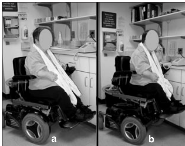
Figure 5 EPW: (a) seat in standard position; (b) seat in elevated position.
