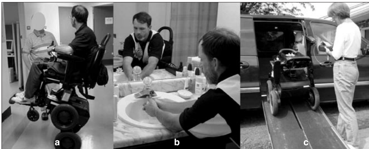
Figure 1 iBOT transporter in use: (a) balance function for eye-level conversation; (b) standard function for washing hands; (c) remote function for loading in a van.
