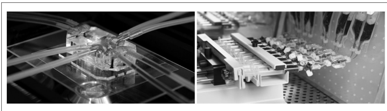
FIGURE 2 Examples of microfluidics (left, printed with permission from the Wyss Institute) and mesofluidics (right, KIYATEC Inc.) “layered complexity” in vitro systems. Both are perfusion based and incorporate 3D microenvironments and coculture interactions, but they differ in scale, manufacturing techniques, potential applications for cell-scaffold constructs, cost, and throughput. These images appear in color in the online posting of this article at www.nae.edu/publications/bridge.aspx .
