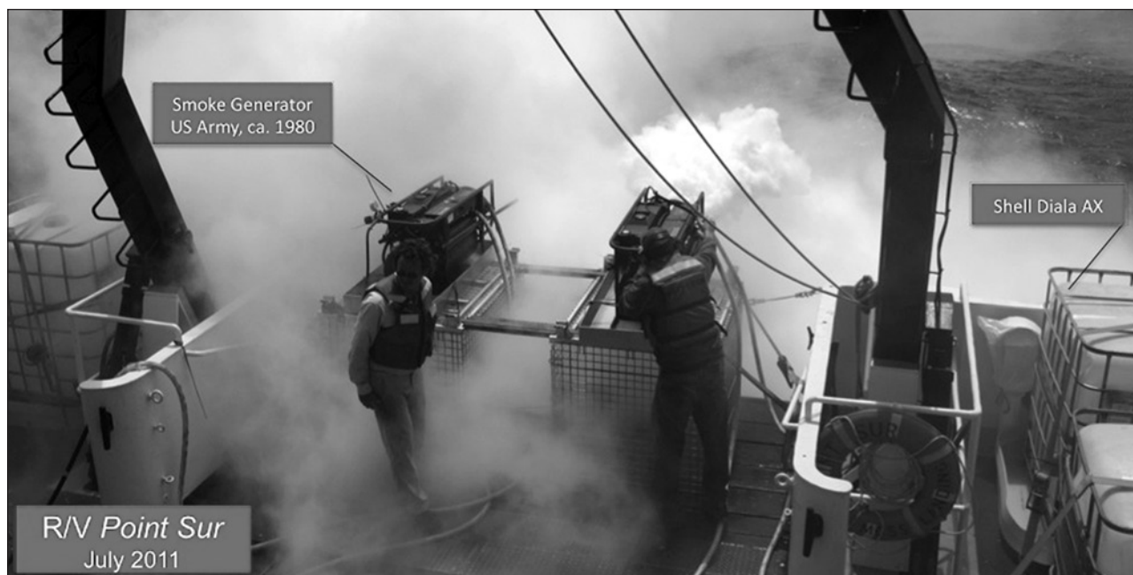
FIGURE 3 Operation of smoke generators aboard the research vessel (R/V) Point Sur for E-PEACE in July 2011. This figure appears in color in the online posting of this article at www.nae.edu/publications/bridge.aspx .
