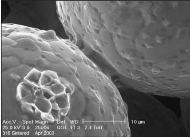
FIGURE 5 Electron micrograph showing a thermal bond produced through sintering to ensure predictable strength and dimensions. Source: Extrude Hone/ProMetal, 2003.
