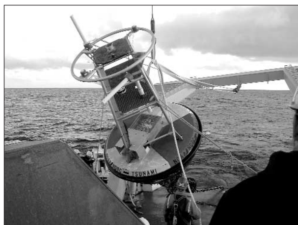
FIGURE 2 A team of NOAA scientists deploys a DART buoy in the Pacific Ocean. In the future, both the Atlantic and Pacific oceans will be covered by 38 buoys that will provide nearly 100 percent coverage for the coastal United States.
