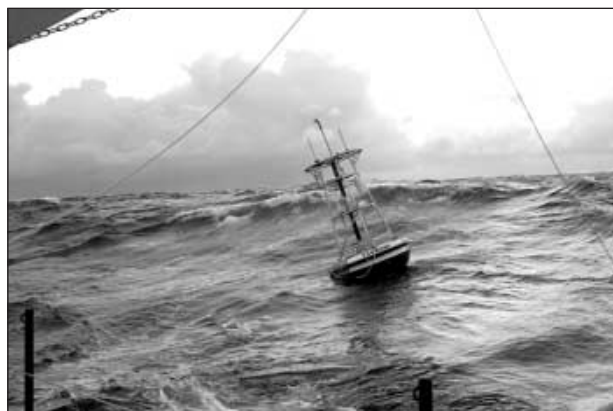
FIGURE 1 A network of DART buoys in the Pacific Ocean that monitors conditions in real time can detect tsunamis with an amplitude of only one centimeter in 6,000 meters of water.
