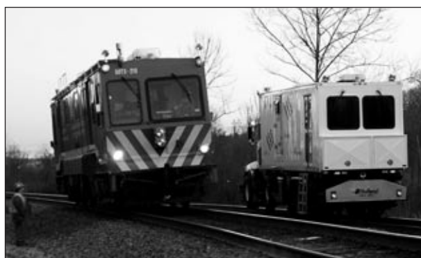
FIGURE 7 Gauge-restraint measuring car (GRMC). The self-contained motorized railcar is on the left; a high-rail inspection vehicle is on the right. Source: Reprinted with permission of Norfolk Southern.
