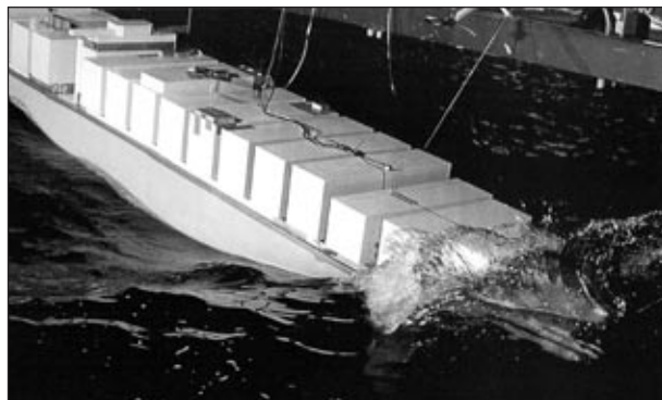
FIGURE 3 Test of a container ship model in extreme head seas. Source: American President Lines. Reprinted with permission.
