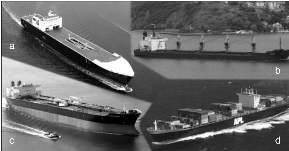
FIGURE 1 Types of ships in the merchant fleet. 1a. Roll on-roll off (Ro-Ro) vessel. 1b. Bulk carrier. 1c. Crude-oil tanker. 1d. Container ship. Sources: Totem Ocean Trailer Express Inc.; EastWind Maritime; General Dynamics NASSCO and BP Shipping; American President Lines. All photos reprinted with permission.
