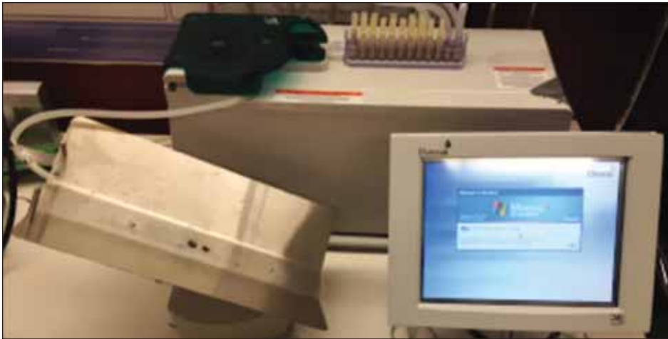
FIGURE 1 An old drug compounder running on a consumer operating system, Windows XP Embedded, was infected with malware, according to a US Food and Drug Administration Manufacturer and User Facility Device Experience (MAUDE) adverse event report in 2010. A former engineer from the company later explained that the malware was accidentally spread to other compounders during the repair. © Kevin Fu.
