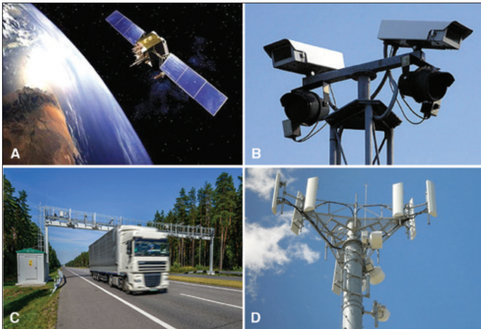
FIGURE 3 Technologies for Automated Collection of Direct User Charges. (A) Satellite Systems. Direct user charges based on mileage rely on GPS technology. Satellites provide location data. In-vehicle equipment receives the latitude and longitude data and uses it to measure travel. Source of image: US DOT Public Roads 69(5). (B) Automated license plate recognition. Reproduced with permission from Adrian Pingstone, Creative Commons. (C) Dedicated Short-Range Communications (DSRC). In-vehicle equipment is activated by DSRC as soon as the vehicle enters the monitoring area and deactivated when vehicle leaves the area. The technology operates in the electromagnetic spectrum's microwave or radio frequency range. Reproduced with permission from TrafficTechnologyToday.com. (D) Cellular Networks. Most roads are within the operating range of cellular networks, which thus represent a promising technology for direct user charging. Reproduced with permission from Telecomtalk, Creative Commons.
