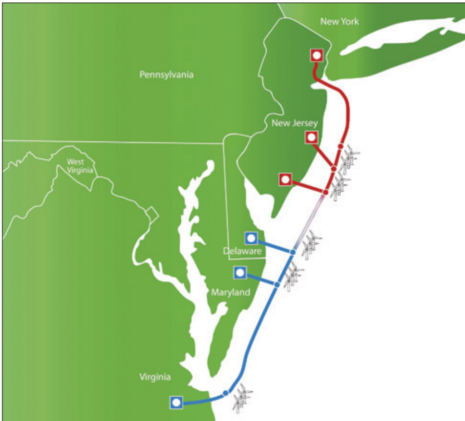
FIGURE 3 Early concept of Atlantic Wind Connection for Virginia, Maryland, Delaware, and New Jersey. Red = phase 1: New Jersey link. Blue = phase 2: Delmarva energy link (Delaware, Maryland, Virginia). Grey = phase 3: Bay link between the phase 1 and 2 connections. Reprinted with permission from Atlantic Grid Development, LLC, available at AtlanticWindConnection.com .
