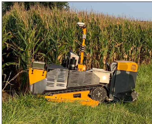
FIGURE 3 Rowbot Systems LLC interrow platform enables in-season fertilization management and cover crop planting before the standing crop is harvested. Reprinted with permission from Rowbot Systems LLC.
