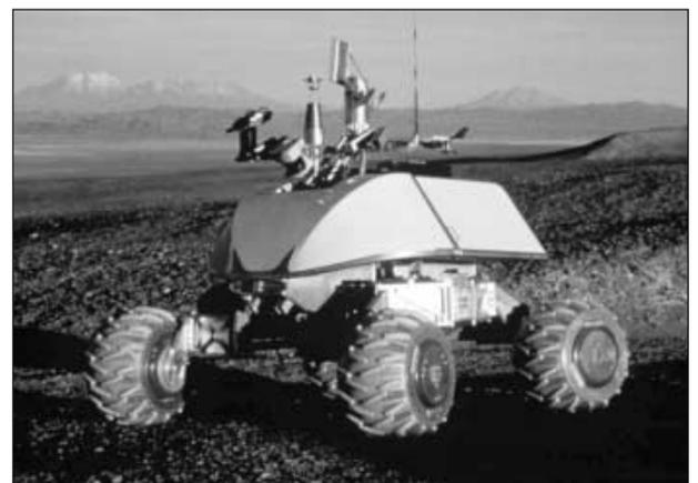
FIGURE 1 NOMAD gasoline-powered robot. Source: Carnegie Mellon University, 2004b.
