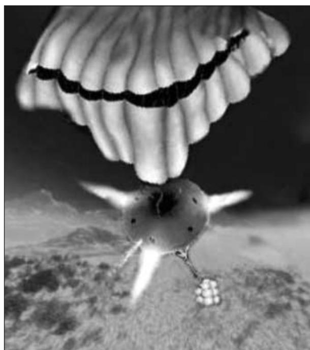
FIGURE 3 Second-generation landing system used on the Mars Pathfinder and MER landers.
