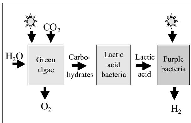
FIGURE 2 A three-stage, continuous, hydrogen-production system. Source: Rechenberg, 1996.
