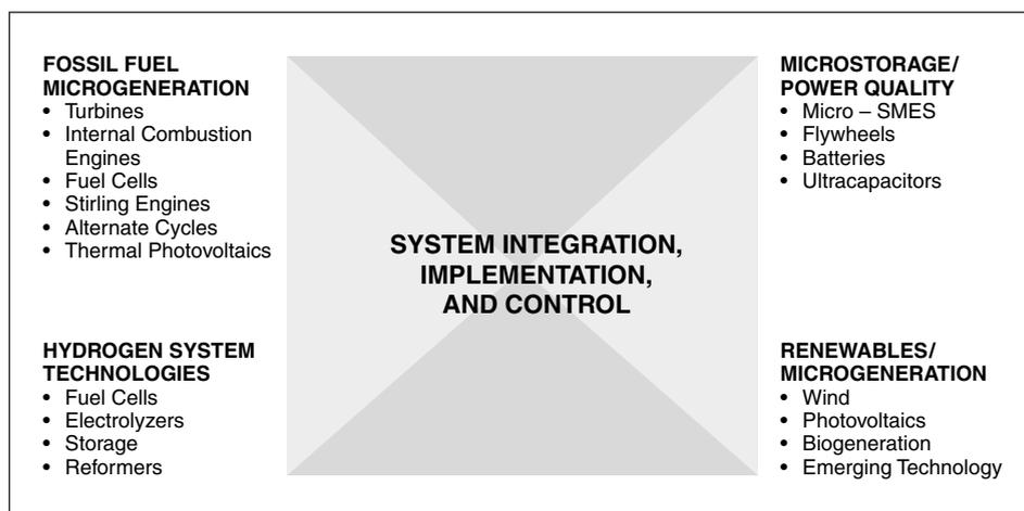
FIGURE 1 Categorization scheme for microgeneration technologies.
