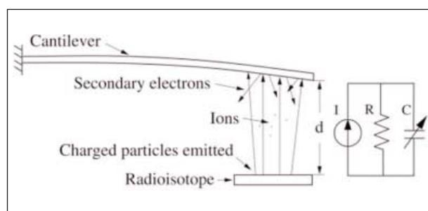
FIGURE 4 Schematic drawing of a self-oscillating cantilever beam. Devices can be modeled as capacitors in parallel with leakage resistors, with most of the leakage resulting from ionization in the gap.
