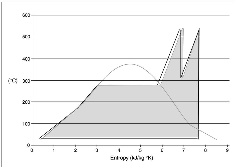
FIGURE 2 Beltracchi display. Source: Burns, 2000. Reprinted with permission.
