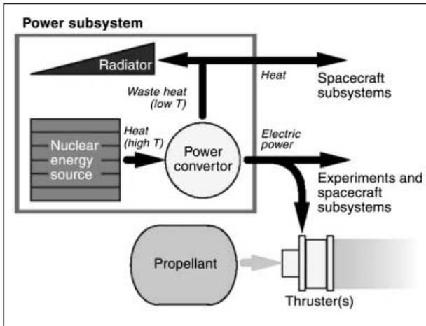
FIGURE 1 Schematic drawing of power flow for a typical nuclear-electric propulsion device. Heat is produced in the nuclear source (typically a fission reactor core) and converted to electricity in the power converter. The electricity is then used to power the thruster. The radiator dissipates the waste heat. Source: NASA, 2001.
