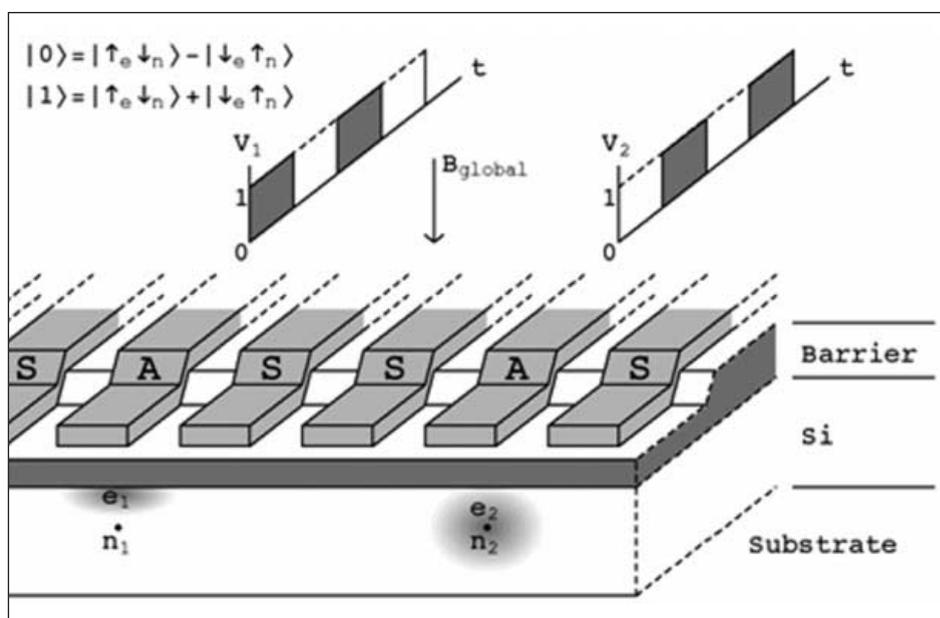
FIGURE 2 Diagram of a silicon-based quantum computer architecture. Single nuclear spins are the qubits; mobile electrons are used to manipulate the nuclear-spin states and move quantum information within the computer. Voltage pulses applied to metal gates on the top of the structure control the positions of electrons inside the silicon.
