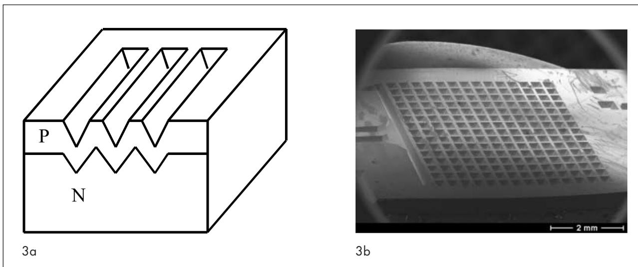
FIGURE 3a A schematic drawing of a simple device using a P-N junction and radioactive source to produce the potential. FIGURE 3b Photograph of a device using pits rather than trenches to hold the source.
