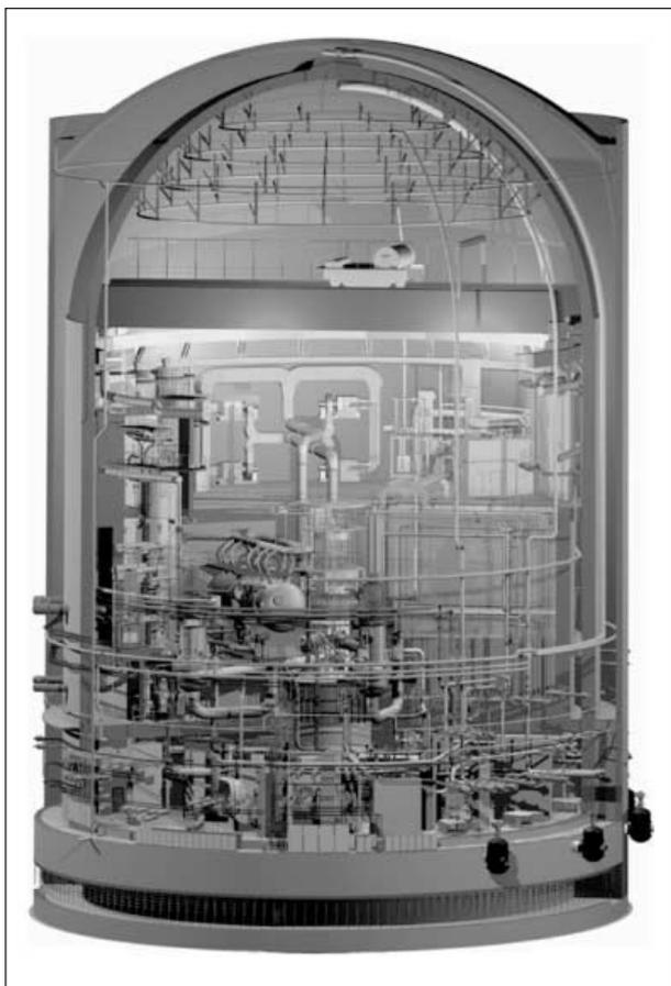
FIGURE 2 Model of 1,000 MW reactor (Lianyungang Unit 1), Elias Mayer, Fortum Engineering, Ltd., Vantaa, Finland. Source: Graphic courtesy of Process, Power and Offshore Division, Intergraph Corporation.
