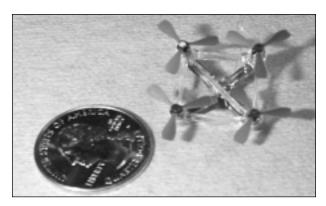
FIGURE 4b Mock-up of the Stanford Mesicopter with four 1.5-cm rotors and a mass of 3 grams.
