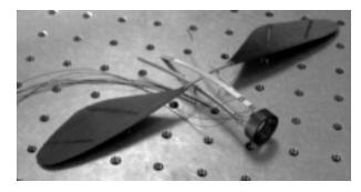
FIGURE 3 Vanderbilt University mesoscale flying robot. Source: Cox et al., 1999.
