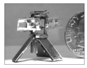
FIGURE 5 Mock-up of the Berkeley micromechanical flying insect (wingspan 25 mm and final mass target 100 mg).
