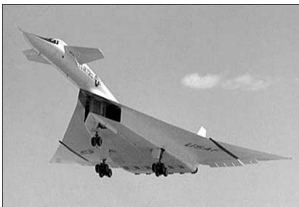
FIGURE 2 The XB-70 was designed to sustain Mach 3. Photo courtesy of [www.fighter-planes.com](http://www.fighter-planes.com).
