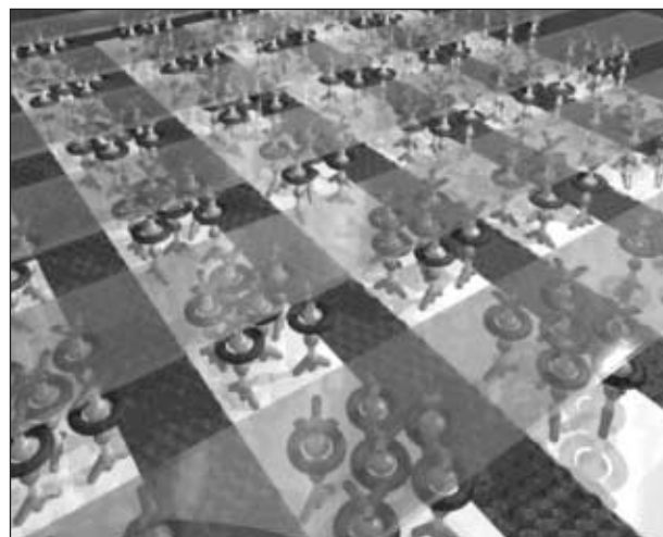
FIGURE 3 A computer graphic showing the molecular components in a crossbar circuit. The [2]rotaxanes molecules shown here are bistable molecular-mechanical compounds. The switching mechanism involves the translation of the ring between two binding sites along the backbone of the molecule. Molecular-electronic circuits have been demonstrated to work as both random-access memory circuits and simple logic circuits.
