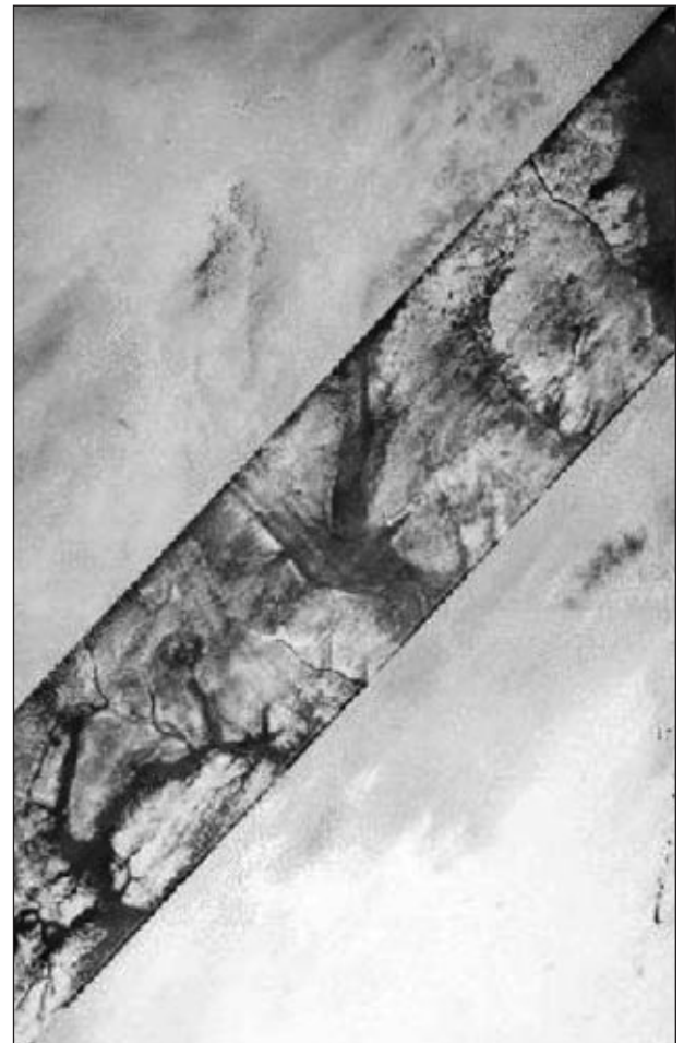
FIGURE 3 A Shuttle imaging radar (SIR-A) strip superposed on Landsat data. The radar waves penetrate the desert sand cover to reveal courses of ancient rivers and streams in an area of North Darfur in northwestern Sudan. Source: Adapted from http://pubs.usgs.gov/gip/deserts/remote/ .
